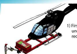
1) First, the Helios HeliMobile is aligned underneath the helicopter at the appropriate recommended location.
