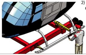
2) Next, the Four clamps are manually secured to clamp the C-Frame of the HeliMobile to the skid frame of the helicopter.
